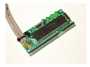
The InterfASD is a keyboard encoder which allows connection of single ended controls to PS/2 keyboard port, then the OS does not need special drivers (also works in DOS).
